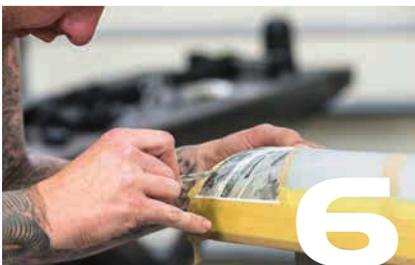
**FASTEN & TRIM:** Apply the graphic over the first panel. Squeegee out any air bubbles that may be trapped. Then use an X-Acto knife to trim the graphic exactly along the inside edges of the green vinyl tape.
