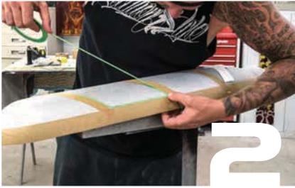
**MASK FOR PANELS:** After the fiberglass “bombshell” is coated with DMD1690 coarse aluminum toner, followed by VM4501 silver flake blended with DBC500 and allowed to dry, an outer panel is marked off using 1-1/2” tape. Four diagonal panels are created using 3/4” tape. The masking provides a guide to run green ProBand Finesline tape along the inside edges. Each end of the shell is masked off as well.
